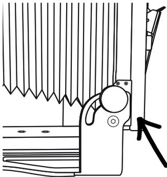
④ Raise front standard and tighten controls.
