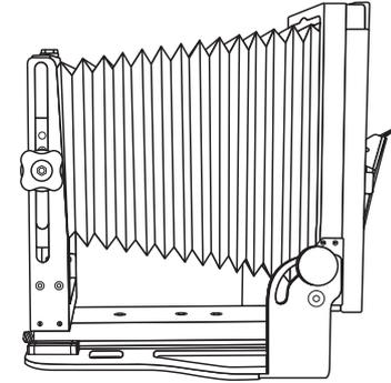
③ Tighten screws and lock rear standard at 90°.
