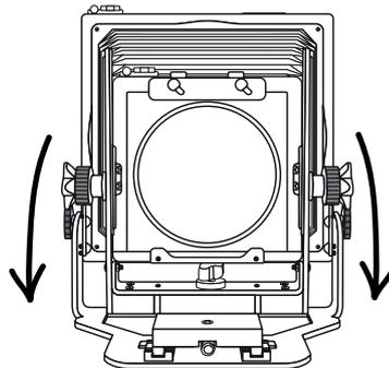
⑦ Tighten rear standard controls to lock camera flat.
