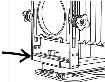
⑤ Loosen rear standard screws on each side.
