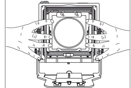
③ Loosen all front standard movement controls.
